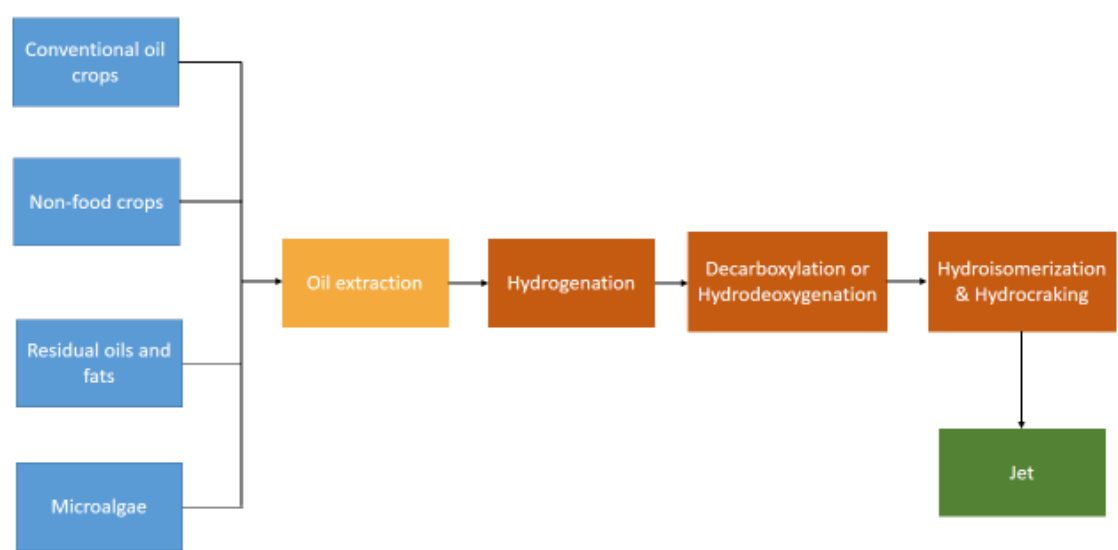
Figure 13: Biomass feedstocks and technological pathway for the HEFA pathway. Based on (GUELL et al., 2012) and (WANG; TAO, 2015)
